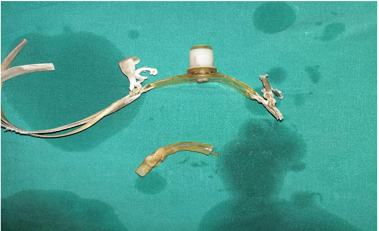
Figure 2. 4.5mm, worn out uncuffed Portex Tracheostomy Tube fractured at the junction of Neck strap and (Bronchoscopically retrieved) Tracheal Part.
