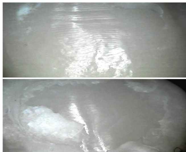
Fig 4: Surface analysis of the bonded surface with Stereo-microscope to calculate Adhesive Remnant Index.
