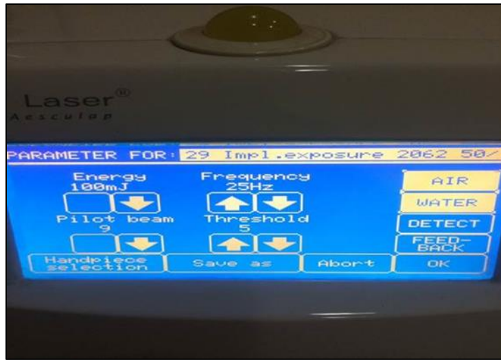
Figure 2. Laser device with the recommended parameters.
